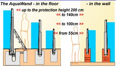
The protective heights of the AquaWand can be selected from 55 cm to 200 cm. The different AguaWand types can be installed in a trench, in a wall or dike can be installed.
